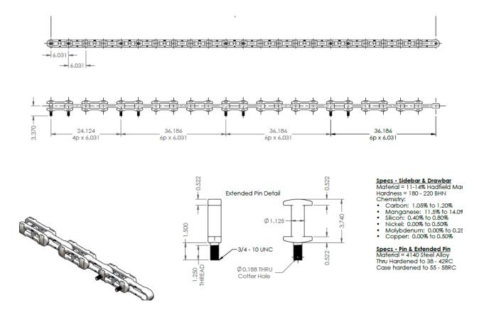
"CXS" Hadfield Manganese Chain is the best choice for this application due to its' ability to endure severe impact. This, combined with the ability to work-harden into the range of 500-600BHN makes this chain an excellent choice for this application. Since installation in May, they have removed only one link and have had zero breaks.
