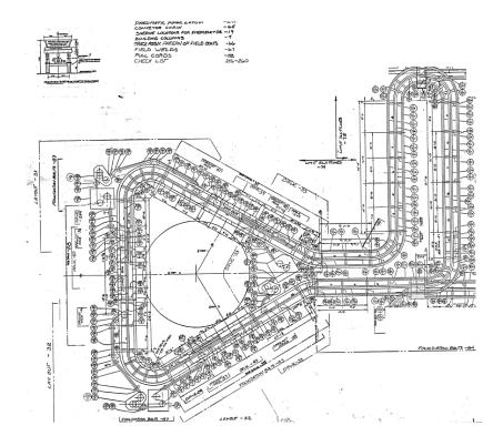
The chain engages a cart which weighs 14,000 pounds and travels at 100FPM. Up to 7 carts can be engaged on the chain at one time.
